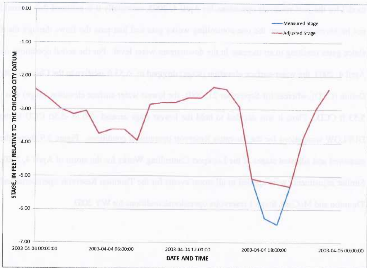
Figure 3.9. Measured stage and stage adjusted to account for the reduction in combined sewer overflows to the Chicago Area Waterway System for the Thornton Reservoir operational conditions for the storm of April 4, 2003.
